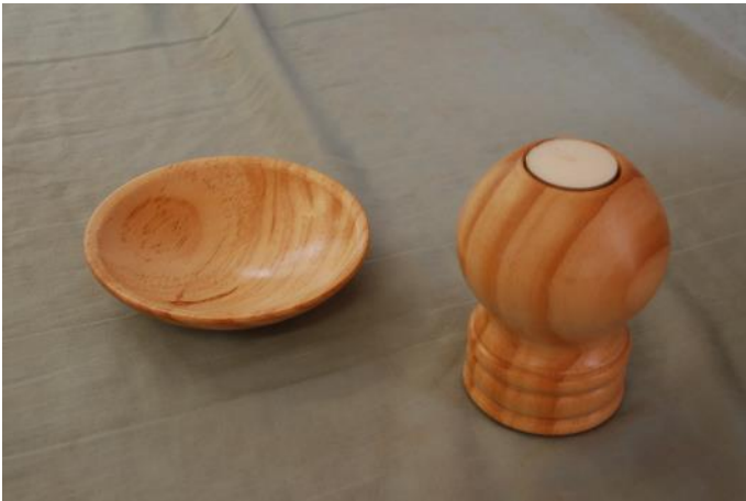
The turned bowl at left and Tea Candle Holder were made by David Keating as part of John Tanner's SIG wood turning course. They are in Pine and finished with EEE and Shellawax. Well done David.
